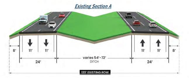
Existing typical section A currently has four, 11-foot-wide travel lanes, with a grass ditch median varying in width between 54 and 72-feet-wide. The existing right of way (ROW) extends approximately 120-feet-wide.
