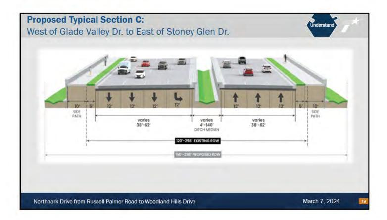
Proposed typical section C would also include six, 12-foot-wide travel lanes with 12-foot-wide left turning lanes at cross streets. There would also be two 5-foot-wide outside buffers and 10-foot-wide side paths in each direction. Proposed ditch medians would be four-to-140-foot-wide with retaining walls constructed to separate the travel lanes and to reduce the impact on existing trees.
