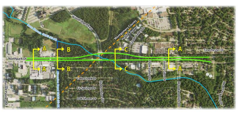
The current layout of Northpark Drive can be separated into distinct sections. The different configurations of these sections are illustrated using typical sections, which are cross-sections of how the roadway looks today.
