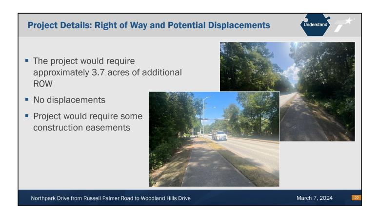
The proposed project would require the acquisition of approximately 6 to 38 feet of right of way (ROW) along the north and south sides of Northpark Drive, resulting in a new ROW width of 126 to 298 feet. The project would require approximately 3.7 acres of additional ROW and would result in 34 partial acquisitions of adjacent property, but no displacements.
