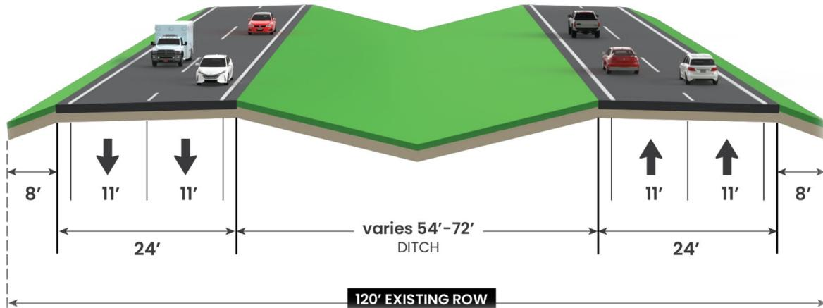
Existing typical section A currently has four, 11-foot-wide travel lanes, with a grass ditch median varying in width between 54 and 72-feet-wide. The existing right of way (ROW) extends approximately 120-feet-wide.
